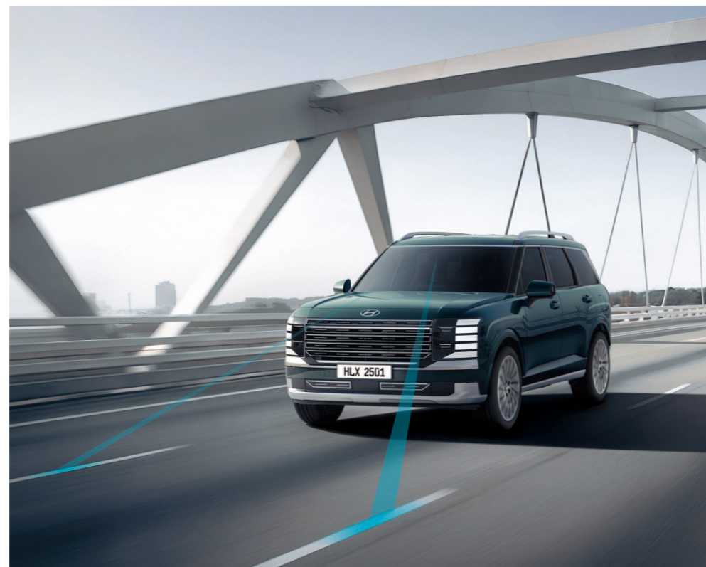
Lane Keeping Assist (LKA) If driving above a certain speed and the driver leaves a lane without the turn signal switch being operated, it provides a warning. When a lane departure is detected, it automatically assists with steering to help prevent leaving the lane.
