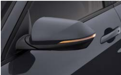
Exterior Sideview Mirrors (heated, power folding, LED turn signal indicators)
