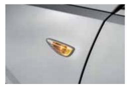
Fender turn signal (Bulb-type, STD)
