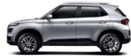
Overall Height (W/ Roof rack) 1,590 (1,617) Overall Length 3,995 Wheel Base 2,500
