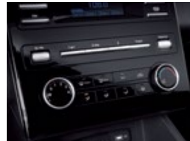
Manual air conditioning system
