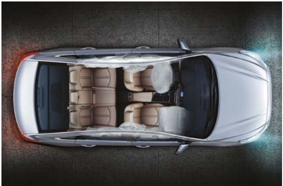
Blind Spot Detection (BSD) Detects approaching vehicles in the blind spot and triggers a warning light and acoustic alert when changing lanes. 6-Airbag system Comprises dual front airbags, two side impact airbags at the front and two curtain airbags running the length of the cabin.
