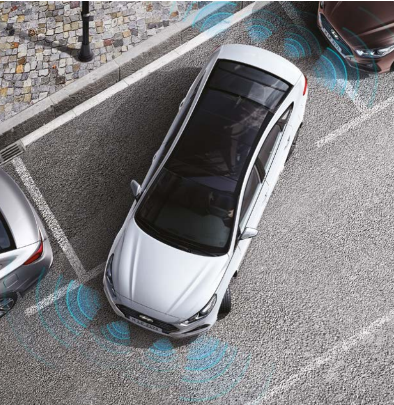
Parking Assist System (PAS) Sensors at the front and rear assist safe parking by activating an audible warning if you get too close to objects when reversing.
