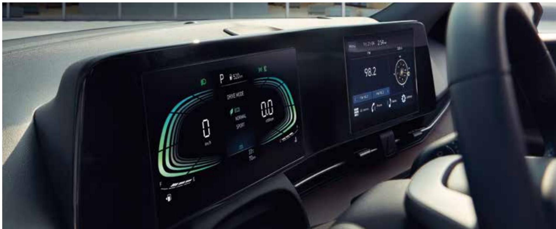
Integrated display audio system and digital instrument cluster
