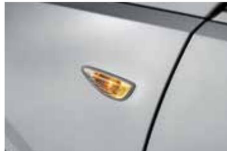
Fender turn signal (Bulb-type, STD)
