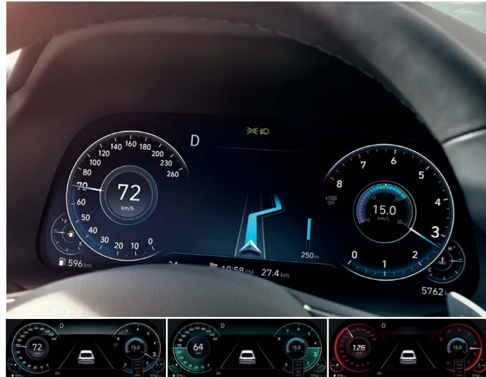
12.3 inch full LCD cluster / Integrated driving mode (Comfort / Smart / Eco / Sport)
