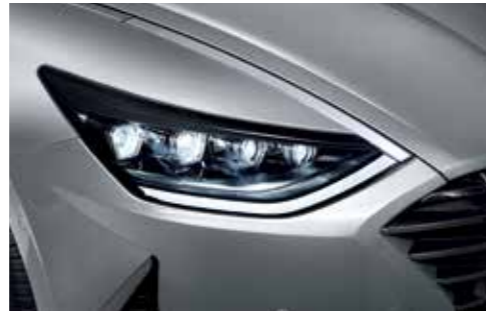
LED headlamps (Projection type) / Daytime running light (LED)
