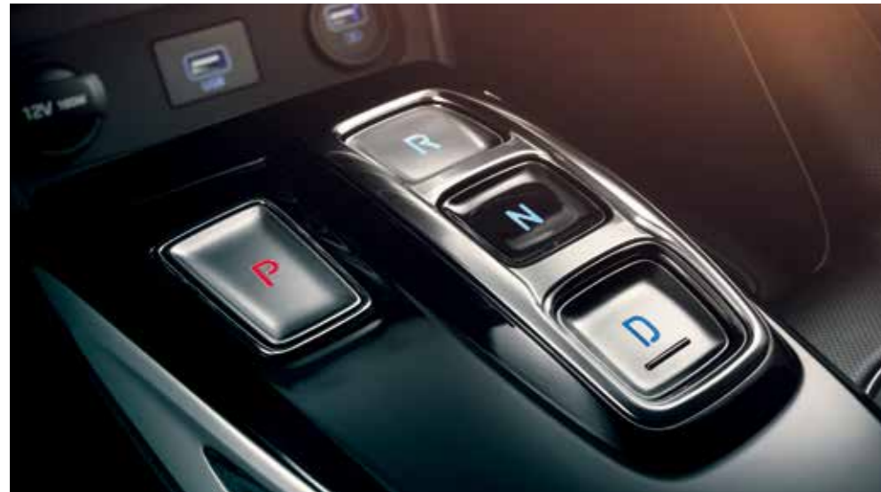
Shift-by-wire automatic transmission
