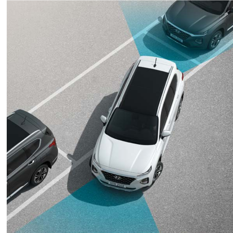
Parking Distance Warning (PDW) Sensors in the front and rear bumpers detect and warn the driver about imminent obstacles for safe parking.
